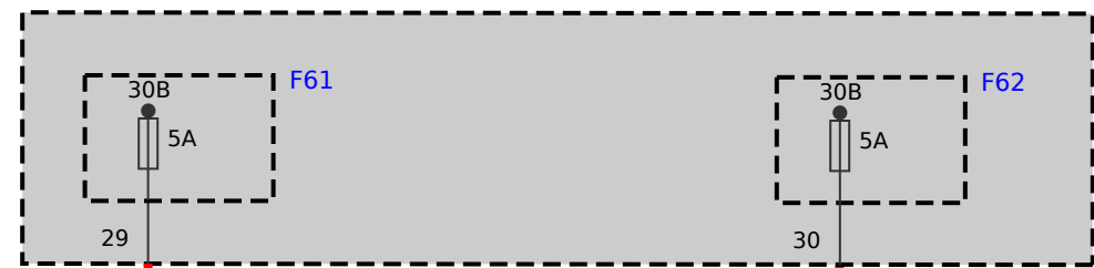
Z44 Front right power distribution box
